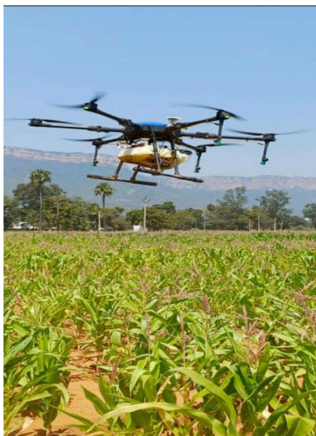
Fig. 1. UAV, ANGRAU- PUSHPAK- 03 drone spraying on maize
