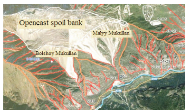
Fig. 3. NTG No. 1–2. Mudflows with dump and dump and extractive types of technogenic landscapes. The NHs associated with them are flow slides and avalanches. Air pollution Legend:
