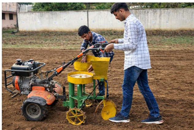
Figure 2. Field evaluation of power tiller operated potato planter
