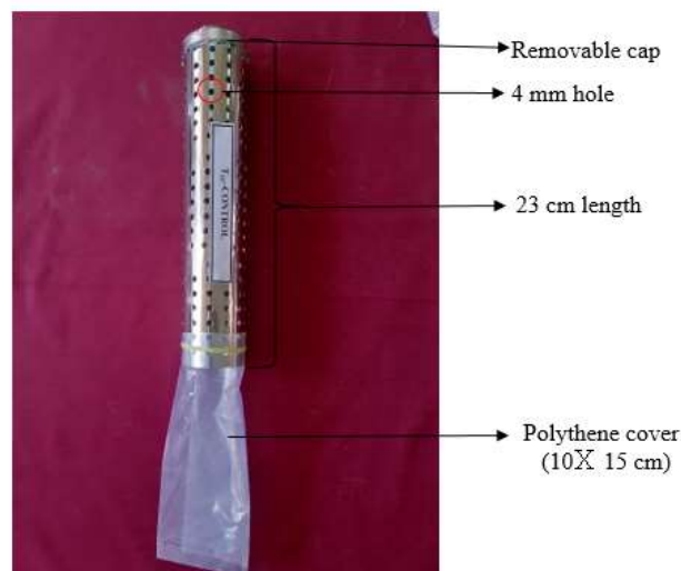
Fig. 1. Structural design of the insect bait trap
