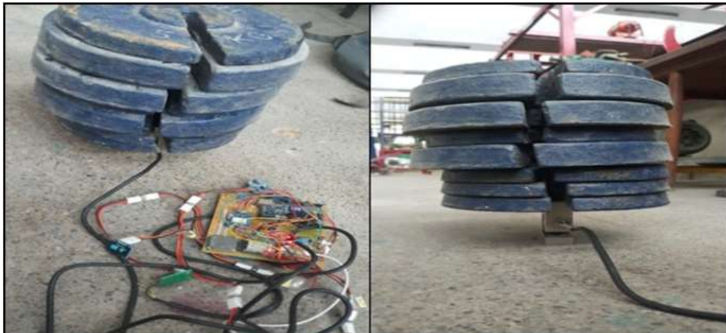
Fig. 1. Experimental setup for load cell calibration with loading and unloading known dead weights
