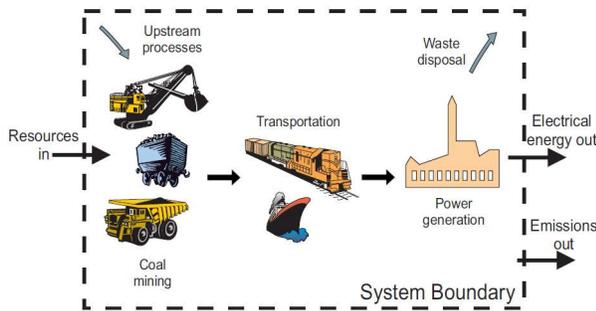
Fig. 6. Systems boundaries for a life cycle analysis of a coal fired power plant (Source: Spath, Mann, and Kerr, p. 4)
