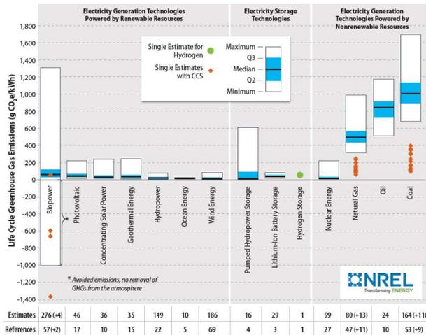
**Fig. 7.** Comparative life cycle greenhouse gas emissions from electrical generation technologies, gCO<sub>2</sub> e/kWh (Source: National Renewable Energy Laboratory, Life Cycle Greenhouse Gas Emissions from Electricity Generation: Update, p. 2)
