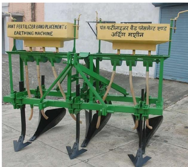
**Fig. 1.** Pant fertilizer band placement cum earthing machine
