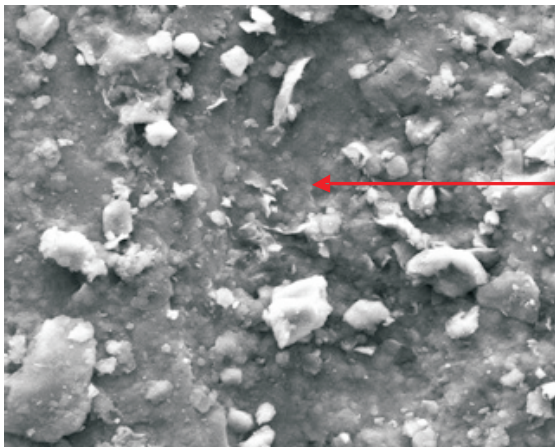
Fig. 4. SEM image of untreated well graded sand
