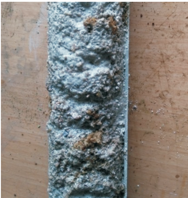
Fig. 6. Soil sample after biocementation process
